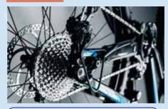
»» Bicycles generally have a chain drive, in which gear wheels of various sizes are connected by a chain.
